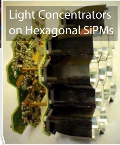
Photon Detection Plane Module
