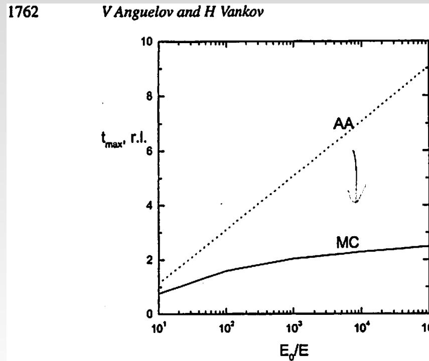
Figure 7. Depth of the maximum as a function of  $E_0/E$ .
