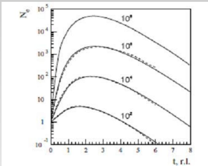
Fig. 11. Cascade curves of electrons for showers initiated by primary electrons in the magnetic field. Different values (indicated at the curves) of the ratio of primary and threshold energies are assumed for the fixed  $\chi_{\alpha} = e_{\alpha}H/H_{cr} = 10^3$ . For comparison, the results obtained in Ref. [24] are also shown (dashed curves).
