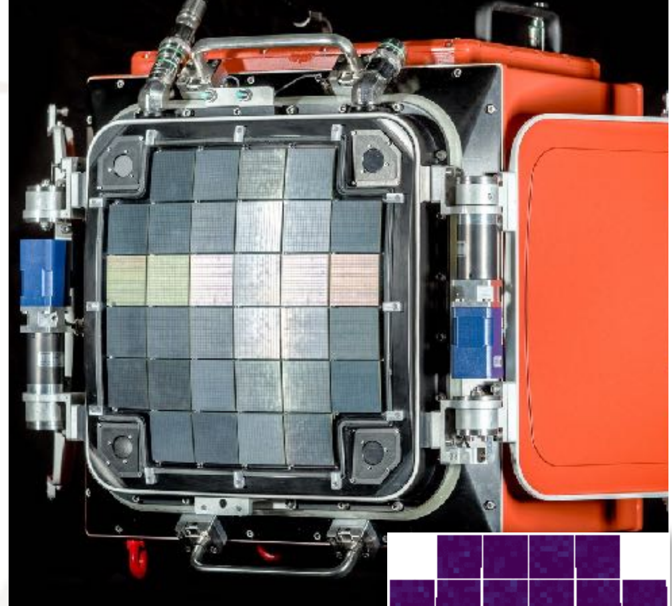
2nd Prototype with SiPMs (First Light 2019)
